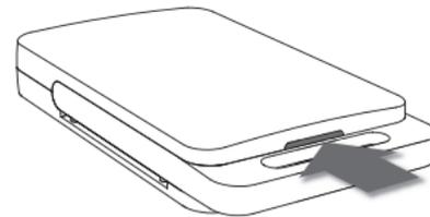
2. Replace the battery. Only use battery type CR2032.
