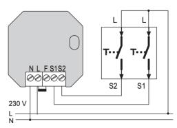
The module transmits telegrams with each change of the switch.
