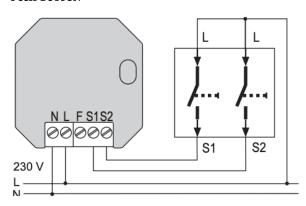
The module transmits telegrams as long as the switch is pressed (up to max. 36 seconds).
