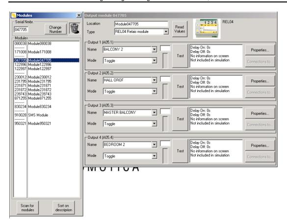
As soon as you write the component's serial number, the right hand side of the programming screen of this particular component will appear. On the upper part of the module's programming screen provides the opportunity to register its location depending on which table it is found and its position on the table. Next, note the component outputs.
