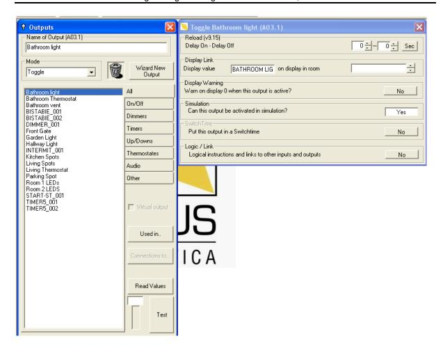
You can also go to the properties of an output directly from the switches in the Modules field of the Serial Manager
