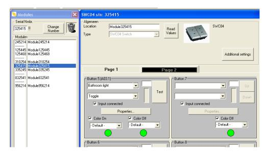
**Attention:** Toggling between pages is done by simultaneously pressing the switch and the 2 buttons. As soon as this is done all 4 keys of the startup's 2<sup>nd</sup> page are controlled. This 2<sup>nd</sup> page selection lasts for 2-5 seconds and then the switch reverts back to the first page startups. You might want to use the second page of a switch for outputs you do not activate regularly (e.g. shutters).
