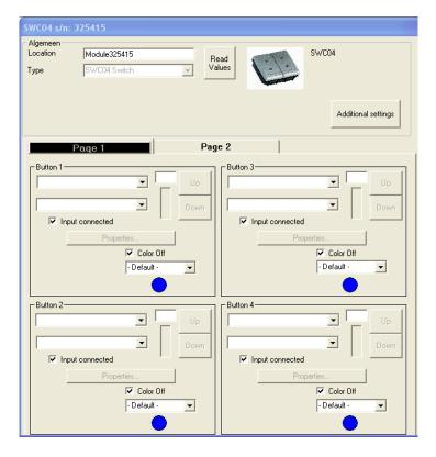
The screen above is the programming screen for a switch where the 4 commands for the switch are displayed. These commands are placed in such a way that the upper left field on the screen (Button 1) will be the upper left side of the switch as you look at the switch, etc.
