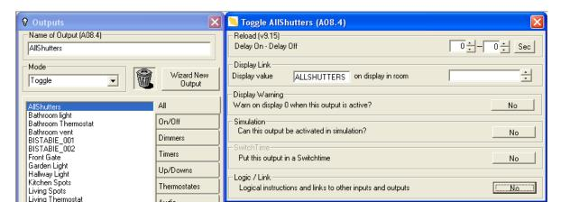
You will be able to select a new multilink – e.g. called AllShutters Multilink, and select all the shutters from the list on the right hand side that you want to control via the same two buttons (one button for up, one for down).
