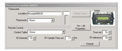
On the first field (location) write the control unit's location in the area.
