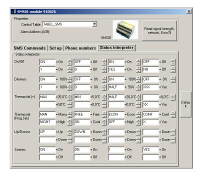
The commands shown above are defined as follows: If you want to turn on a relay contact (on/off) all you have to do is write the contact name as it was entered in the "sms command" tab then insert a space and write ON or 1 or YES as the following table shows. Similar procedures are used for dimmers, blinds, etc.
