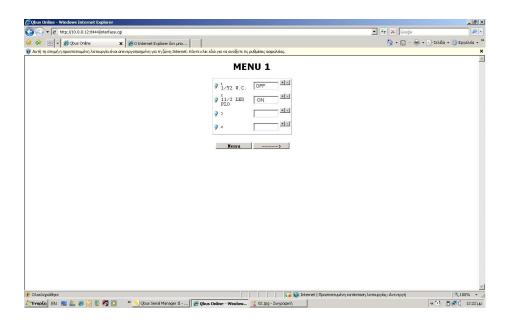
Each menu is comprised by more than one page depending on the amount of controlled elements. Using the  $\rightarrow$  key, you can move to the next page while with the menu button you can come back to the initial menu screen.
