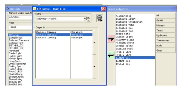
Now all that's left is to allocate the AllShutters Fictive output to a switch – using the pushbuttons on that switch you will be able to control all shutters at the same time.
