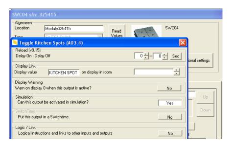
Reload: add a delay for activating or de-activating the selected output (delay between when you push the switch and the (de-)activation of the related output.
