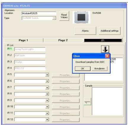
You will see the date and time of the samples you created. By clicking on that date and time stamp you will see the 12 samples individually appearing in the box called "Sample" on the IR page. Double-clicking each sample will cause it to be allocated to the Output in the IR List that is highlighted in green.
