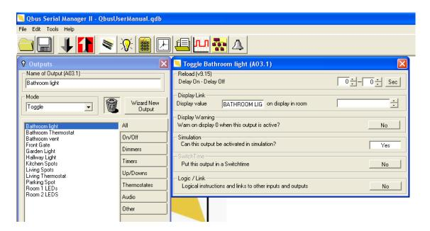
Once you have selected all outputs you want to be activated in a simulation, you can check that list by clicking on the "Edit"-button, then on "Simulation" which will give you a screen that will contain only those outputs that have been selected to be activated in a simulation.
