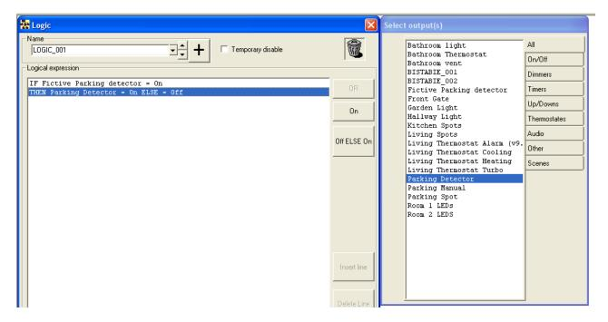
• Step 3: in the MDI or MDO, use the fictive output as one of the controlled output: now when the MDI will detect something, it will turn on the fictive output which will on its turn activate the Timer 5 Detector part (as both are linked through logic).
