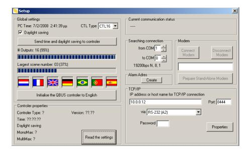
When you try to install the first communication, it will search first for the IP address and then for the COM ports. The indicator "TCP/IP active" will be displayed on the upper right side of the screen.
