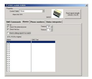
Setting up the alarm for SMS, in order to receive also a text notification, is done as follows. Go to the SMS module through the modules option on the program command like and then choose the alarms tab; the following screen will appear.
