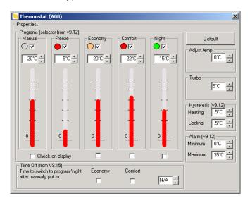
This screen shows 4 thermostat programs and the manual operation. By clicking the fields right underneath the program names, you can select which programs you want to control from the thermostat.
