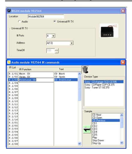
Next, you need to select the Device Type you want to control (you will need to sample the infrared codes you want to use in to the Qbus system first according to the instructions given under "Sampling IR Codes"), and then double-click on the samples to link them to a specific port and code. You can enter a name in the IR Function.
