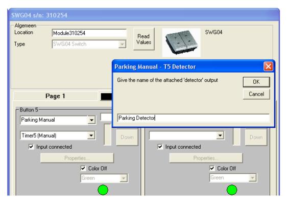
Step 2: you need to link the Timer 5 Detector part to the detector you will use to control this
