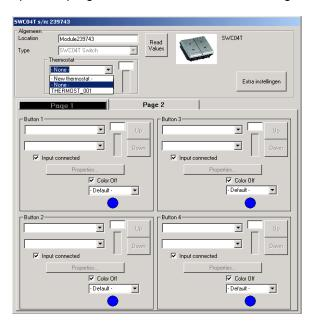
Note that besides the two fields on the upper part of the screen, the switch location is mentioned along with the type and a third field that has to do with the thermostat. This way you can add a new thermostat or to use one of the ones already made. The thermostat settings are the same with those mentioned for the THI.
